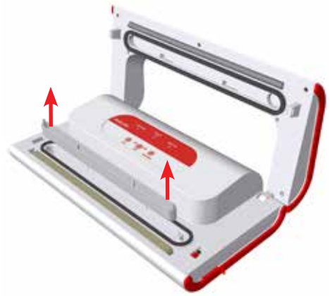
Figure 6: When liquid finds its way into the vacuum channel, lift the Liquid Trap tray directly upwards, pour the liquid out, wash the tray, and dry it thoroughly.
