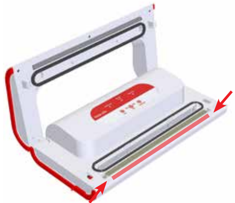
Figure 3: Adhere Status Stiki tape next to the Sealing Strip.
